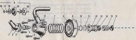
STEP 2-Assemble control valve parts 10 through 15, into end plate. Securely tighten fitting (12). On Hydrovaes with double atmosphere poppet, assemble group "A" parts in to housing (6) as a sub-assembly. For replacement of control valve poppets in other Hydrovacs, see reverse side. Attach remaining parts 1 through 9 to end plate.
