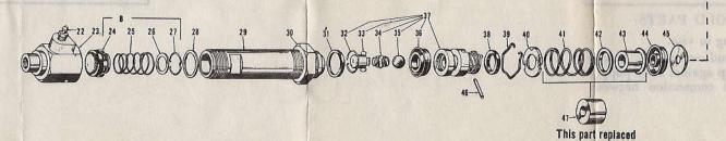
STEP 3-Assemble new type stationary seal parts 39 through 45 into center bore of end plate. Discard stationary seal retainer (47). Assemble end seal (38) in against shoulder of end plate. Assemble hydraulic piston parts (32) through (37) as a subassembly. Assemble parts (23) through (31) as a sub-assembly. Securely tighten cylinder (29) into end cap (23). Note: Group "B" parts not used in all Hydrovacs.
